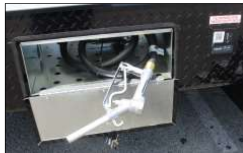
40-Gallon Fuel Station
