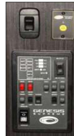
Centralized Monitor, Lighting & Inverter Controls
