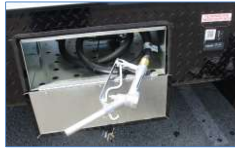
40-Gallon Fuel Station
