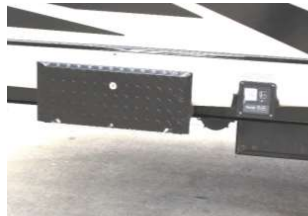
40-Gallon Fuel Station
