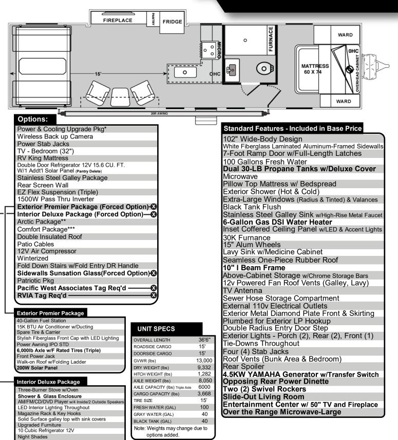
Power & Cooling Upgrade Pkg\* Includes 6.0KW Yamaha Generator Upgrade, 13.5K BTU Bedroom A/C(w/wall control), 50 Amp Service
