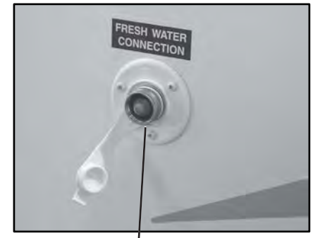
City water connection - note filter screen ( color and style varies with model )
