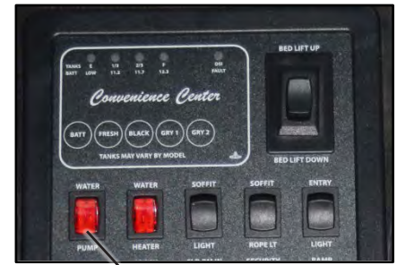
Water pump switch on Convenience Center panel
