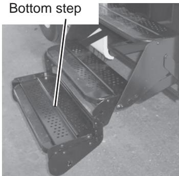
3. Fold the bottom step down. Be sure bottom step is unfolded completely.
