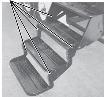
4. Reverse the procedure to retract. Be sure the step assembly is secure.
