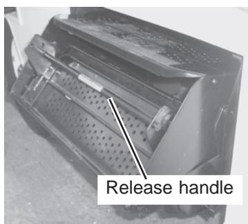
1. Grasp and pull up and out on the release handle under the top of the step assembly. Pull step assembly out from trailer body. Grasp and wiggle the step to be sure it is completely extended and locked in position. (Step is shown partially extended.)
