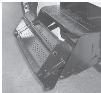
2. Rotate the step elements out and downward.
