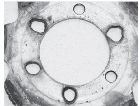
This wheel was operated with four loose wheel nuts. Note the damaged holes, and that only two nuts were holding the wheel on the axle hub.
